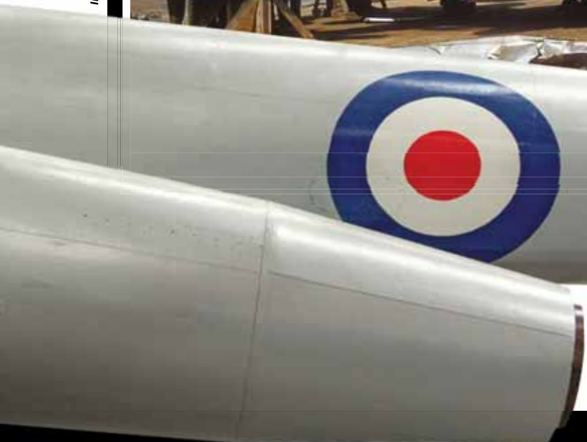
The FR.9 was a basic F.8 airframe, with only the camera compartment in the nose being different
